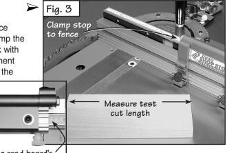
`Slide scale to read board's ' length under either end of stop
