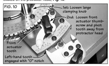
Rotate the protractor head to the desired angle, then firmly engage the tooth on the front actuator with the corresponding notch on the protractor head. The actuator tooth should point directly to the desired angle on the scale. Tighten the large clamping knob, then tighten the front actuator thumbscrew, **Fig. 11**.
