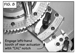
Now pivot the rear actuator to engage the right-hand tooth with the notch marked "CAL" on the rear scale, **Fig. 9**. If adjusted properly, it will pivot perfectly into the notch. To adjust, loosen the
