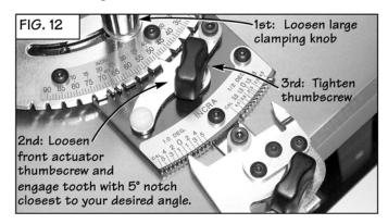
Loosen the rear actuator thumbscrew. Use the left-hand tooth to add or subtract from the coarse adjustment setting in 1° intervals. Use the right-hand tooth to add or subtract from the coarse adjustment setting in 1/2° increments. Engage the tooth firmly in the selected notch, then tighten the large clamping knob and the rear actuator thumbscrew, **Fig. 13**. **Important:** After completing your cut, don't forget to return the rear actuator setting to the 0° notch.
