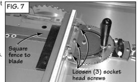
This one-time calibration prepares your INCRA Miter 3000 for work in either miter slot. Just remember that the accuracy of the INCRA Miter 3000 at any subsequent setting is dependent upon the accuracy of your initial 90° calibration. Verify this important calibration with a test cut and fine tune as necessary.
