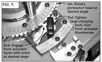
**Caution:** After making any adjustments to the miter angle of your INCRA Miter3000, always <u>verify safe</u> <u>clearance</u> between the fence and the blade <u>before</u> turning on the saw.
