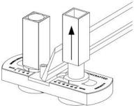
Raise the sleeve to expose fresh abrasive. Flip end for end to expose even more abrasive.
